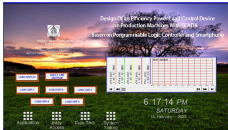
Figure 12. HMI display when connected to PLC
