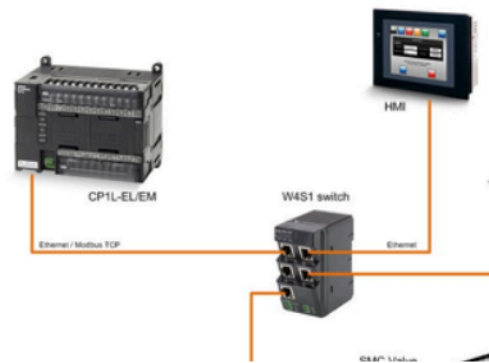
Figure 5. Communication cable connection between Omron CP1L PLC and MTV via HUB
