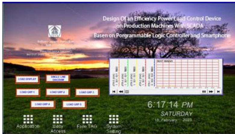
Figure 12. HMI display when connected to PLC
