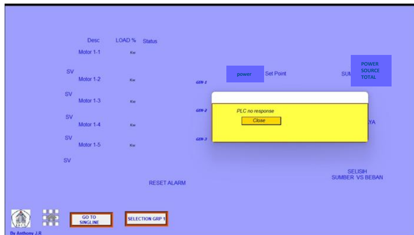
Figure 11. HMI display indicator that is not connected to the PLC
