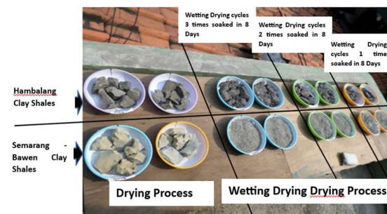
Fig. 1 Changes in the physical properties of Semarang-Bawen and Hambalang clay shale due to the drying process and the drying wetting cycle (Alatas I M 2015 d)
