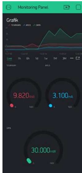
Figure 9. Display of the designed BLYNK application
