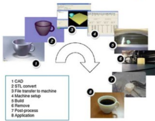
Fig. 1.2 Generic process of CAD to part, showing all eight stages
