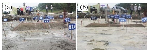
Figure 17 Differential settlement of embankment on the liquefaction site: (a) before blasting; (b) 30 min after blasting.
