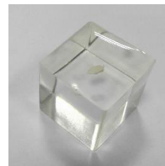
Figure 2. Calcareous sand particle cubic specimen
