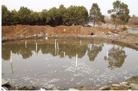
Figure 6 Layout of single shallow-buried detonation tests
