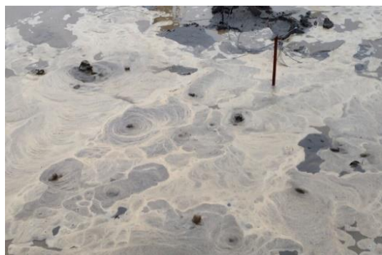
Figure 13 Large area of sand boils in the test site
