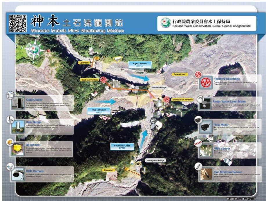
Figure 1. The monitoring layout of Shenmu Station [2].
