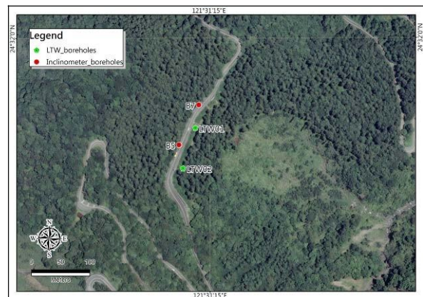
Figure 4. Locations of the investigation boreholes and inclinometers.
