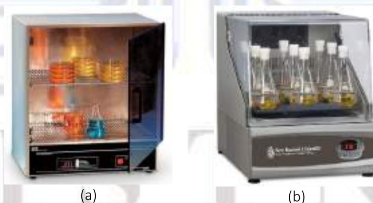
Gambar 2.7 Ruang kultivasi. (a) Inkubator statis; (b) inkubator bergoyang (sumber: www. Generasibiologi.com ; https://us.vwr.com/ )
