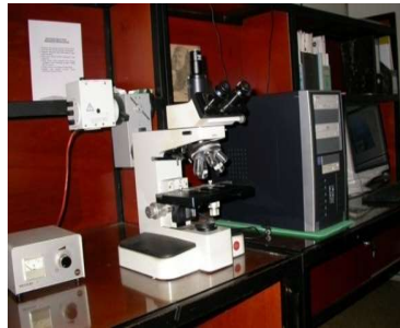
Figure 3. Optical Microscope for Metallographic Test Equipment
