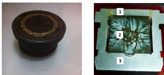
Figure 2. Holding Magnets and its parts (1. Cu; 2. Magnets; 3. Steel)
