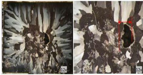
Figure 9. Magnet micro structure, there is a porous defect in the middle area and cracks through the grain boundaries (intergranular crackings) in the form of ferritic and fine carbide grains spread evenly. (Etching: K_2CrO_7 )
