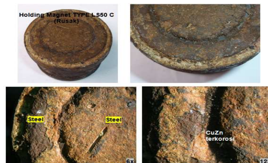
Figure 16. Macro photo of Holding Magnet LS50 C
