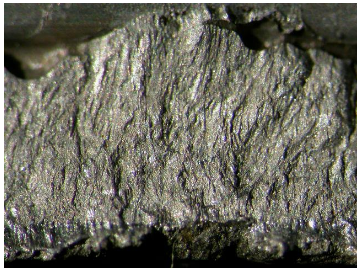
Weld defect (gas porosity)
