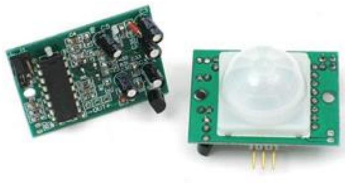
Gambar 2.12 Gambar Sensor PIR HCSR501
