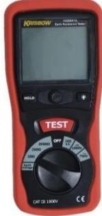
A handheld digital earth tester with a red and black body. It features a small LCD screen at the top, a 'TEST' button, and a rotary dial with various settings. The bottom of the device has a 'CE' mark and 'OUT 110KV' text.                           |
