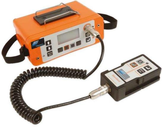
The image shows a cover meter test kit. It consists of an orange rectangular control unit with a digital display and several buttons. A black coiled cable connects this unit to a smaller, black rectangular probe. The probe has a small display and buttons on its top surface.                                                                                   |
