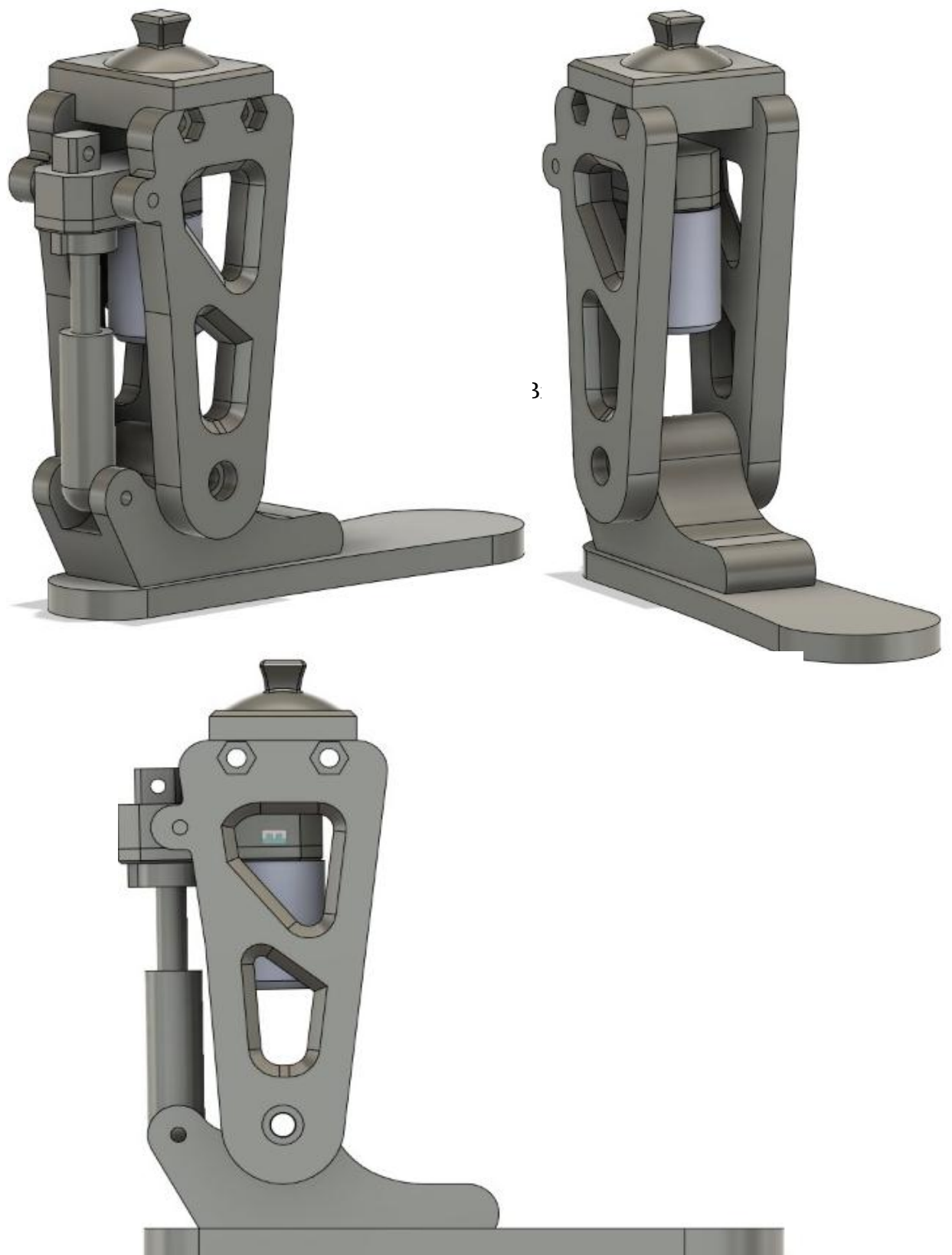
Gambar 4.11 3D model Transtibial Bionic Prosthesis dengan Software Autodesk Fusion 360
