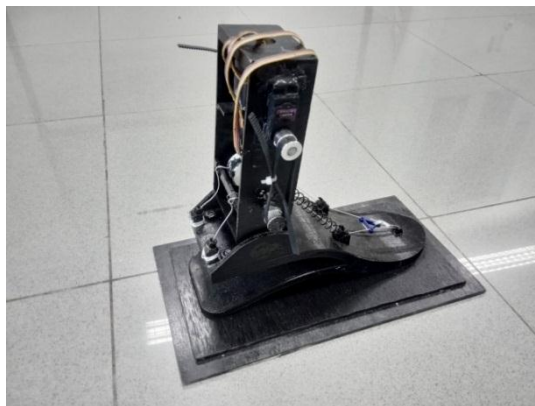
Gambar 2.20 Transtibial Bionic Prosthesis penelitian pertama
