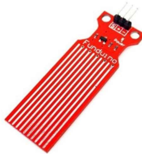
Gambar 3. 9 Hardware Sensor Water Level
