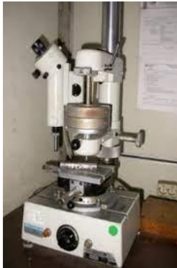
Gambar 3. 7 Alat uji kekerasan Vickers hardness tester (frank finotest)
