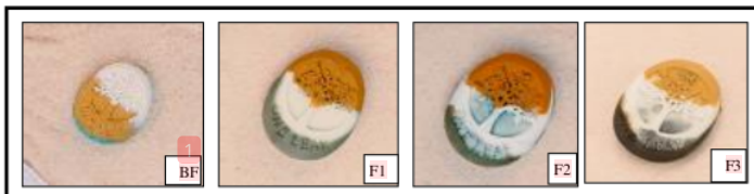
Figure 1. Solid bar soap formulation. BF: basis formula; F1: formula with 1% oil palm leaves extract; F2: formula with 2% oil palm leaves extract; F3: formula with 4% oil palm leaves extract.
