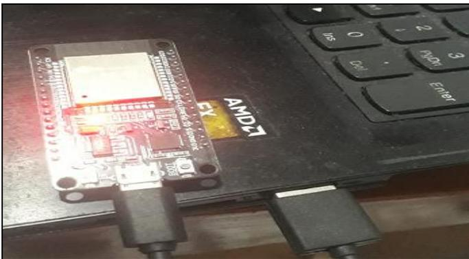
**Gambar 30.** Proses Upload ke Board NodeMcu Esp32 DevKitV1
