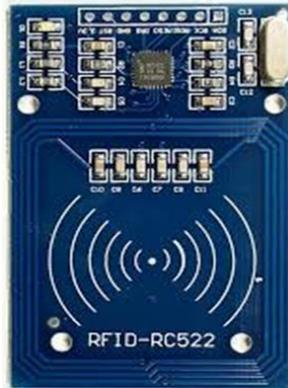
**Gambar 18.** RFID Reader RC522
