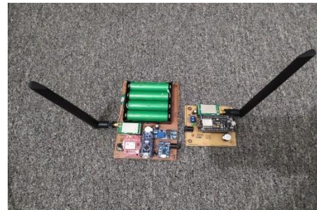
Gambar 25 Transmitter dan Receiver
