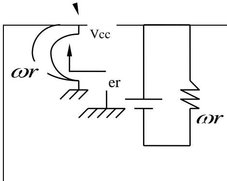
$$e_R = \frac{R_{\omega r}}{R_{tot}} \times V_{cc} \dots \dots \omega r_{min} = 0$$
