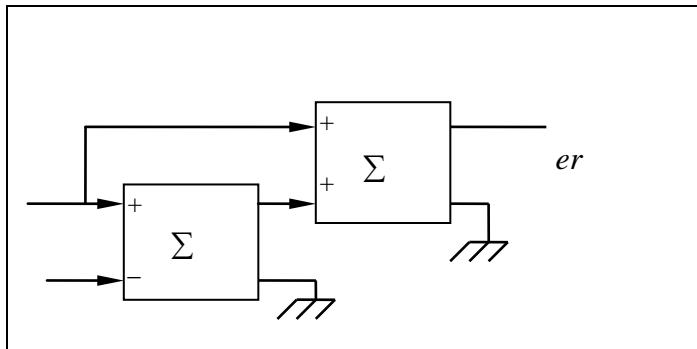
$$\begin{aligned} e(t) &= el(t) + er(t) \\ el(t) &= er(t) - e_{TC}(t) \Rightarrow \\ e(t) &= 2er(t) - e_{TC}(t) \\ TL \rightarrow E(s) &= 2Er(s) - E_{TC}(s) \dots\dots(2) \end{aligned}$$
