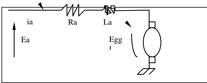
$$\begin{aligned} ea - egg_1 &= Ra \cdot ia + la \cdot dia/dt \\ Ea(s) - Egg_1(s) &= (Ra + LaS)Ia(s) \\ \frac{Ia(s)}{Ea(s) - Egg_1(s)} &= \frac{1}{LaS + Ra} \dots\dots(4) \end{aligned}$$
