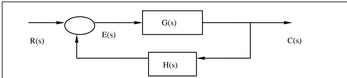
$$E(s) = R(s) - H(s).C(s) \dots\dots\dots(1)$$
