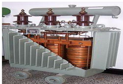
Gambar 5.1: Transformator Daya
