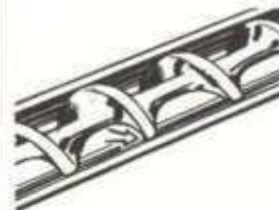
3. Revolving Worms and Spirals in Enclosures
