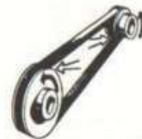
9. Pinch Point Between Belt and Pulley Wheel
