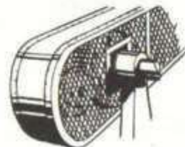
6. Pinch Points Between Two Revolving Parts
