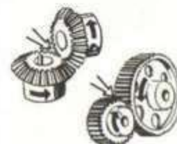
6. Pinch Points Between Two Revolving Parts
