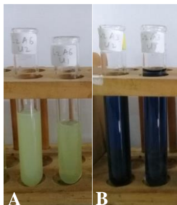
Figure 2. The Reaction Between Gallic Acid and Folin-Ciocalteu reagent. A. Before adding NaOH, B. After adding NaOH
