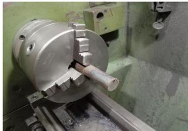
**Gambar 4.11** Posisi As Pendorong Di Mesin Bubut
