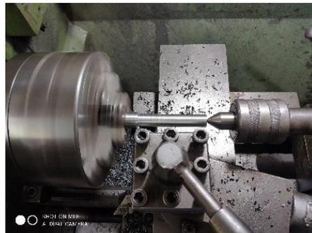
**Gambar 4.15** Proses Pemakanan Samping As Pendorong
