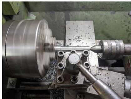
**Gambar 4.14** Proses Pemakanan Samping As Pendorong
