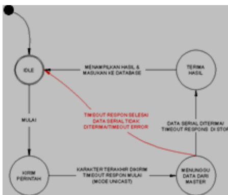
Gambar 3.6 Diagram keadaan HMI / Scada Monitoring
