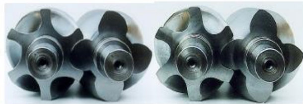
Fig. 3 Comparison of Asymmetric Rotors (left) and 'N' Rotor Replacement (right)
