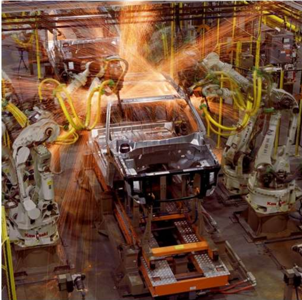
Figure I.13 Automated spot welding of automobile bodies in a mass production line. Source: Courtesy of Ford Motor Company.
