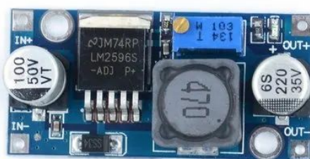
Gambar 2. 19 Step down dc LM2596
