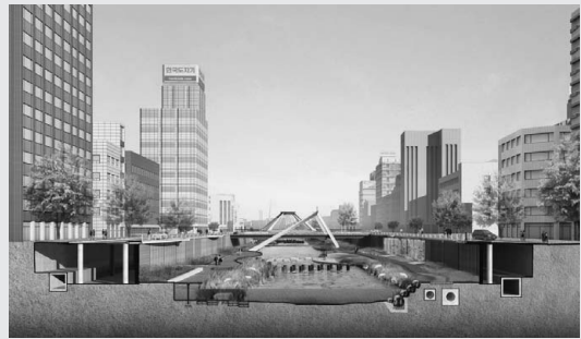
Figure 8.15 Schematic diagram of Cheonggyecheon restoration project, showing infrastructure as well as the river.
