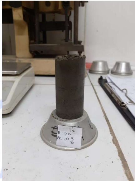
Compaction PC 10% 20 B/L
