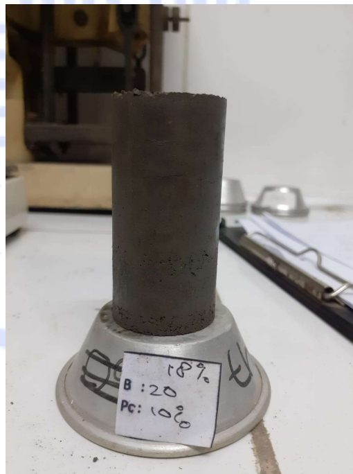
Compaction PC 10% 20 B/L
