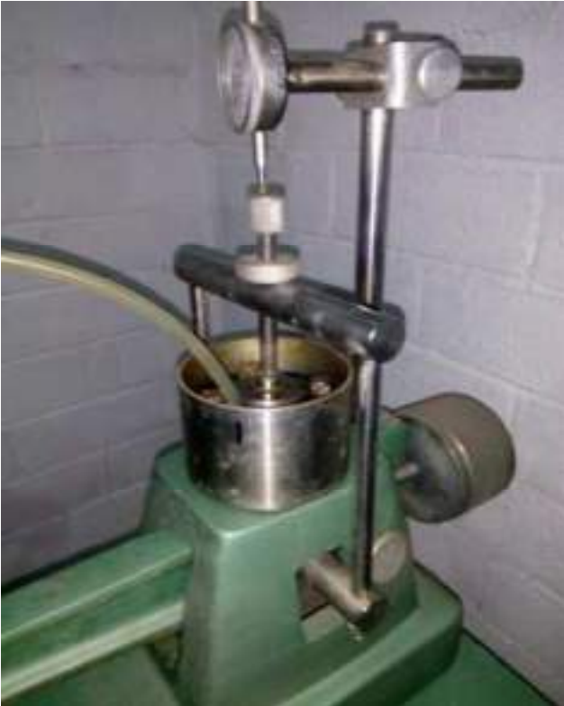
Dewatering after finished Cycle 1
