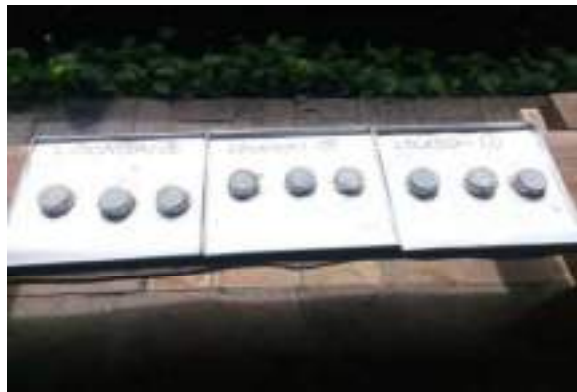
6 hours natural drying before in to Oven
