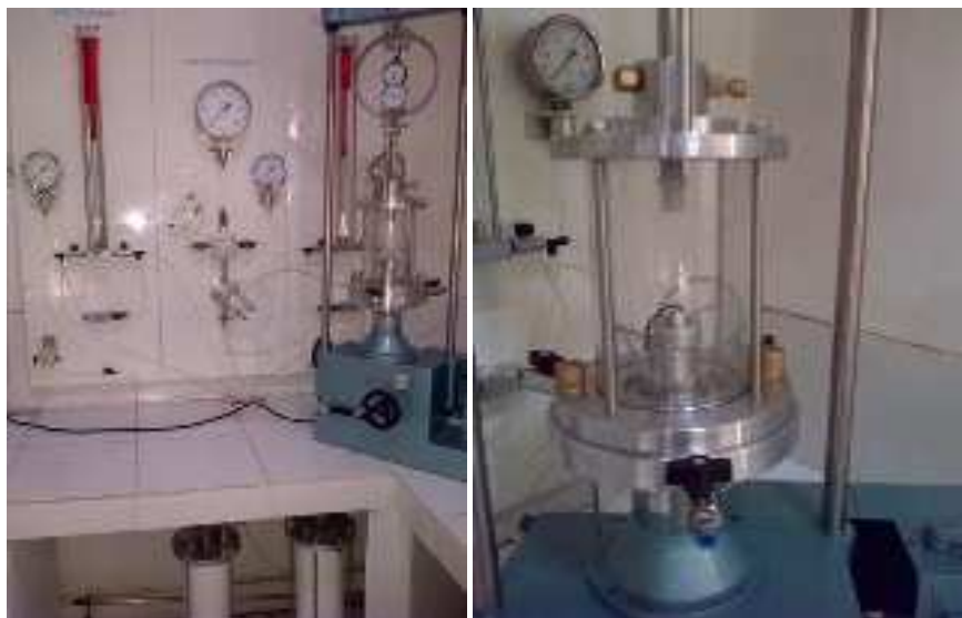
Gambar L 1 Peralatan uji tri-axial di makmal Geoinves, Jakarta, Indonesia
