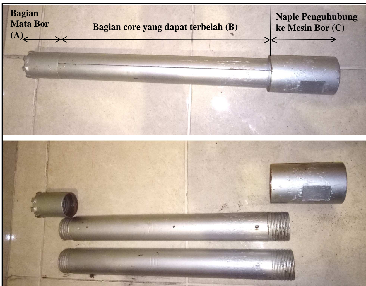
Gambar 3.3 Split Single core barrel / baru
