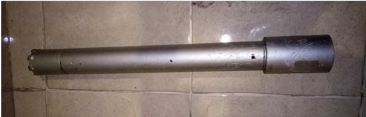
Gambar 3.2 Single core barrel (lama)
