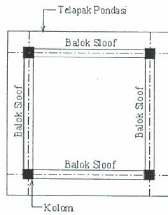
Gambar 2.8 Pondasi full plate (Tampak atas)
