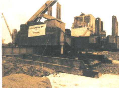
Foto Pelaksanaan Axial Loading Test Pile No: 450A Ondo Metal New Factory
