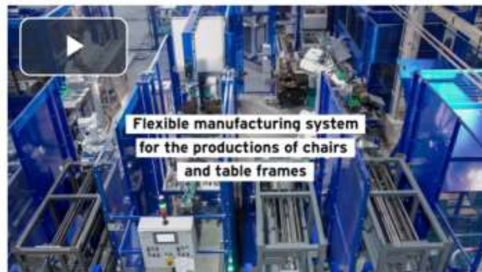
Flexible Manufacturing System with multiple pallets storage five axis machining: N. 1 THS 100 X - N. 3 Roller XL
