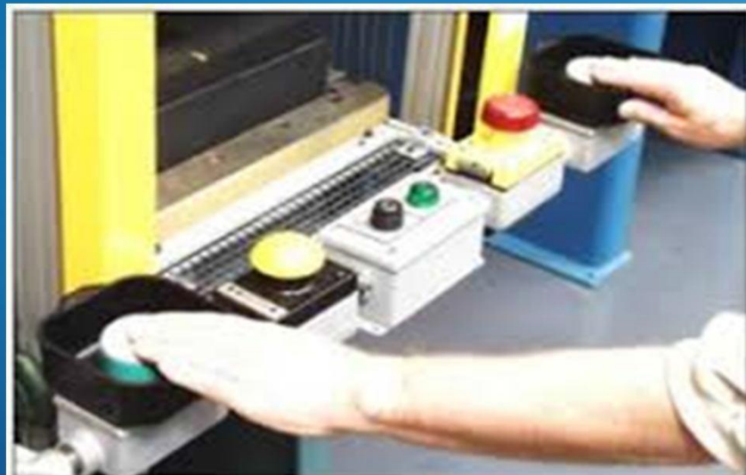
Two-hand Control on a Press
