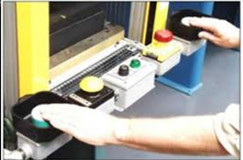
Two-hand Control on a Press
