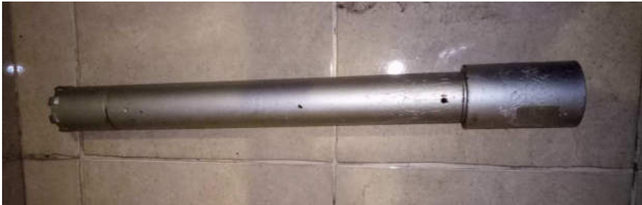
Gambar 3.2 Single core barrel (lama)
