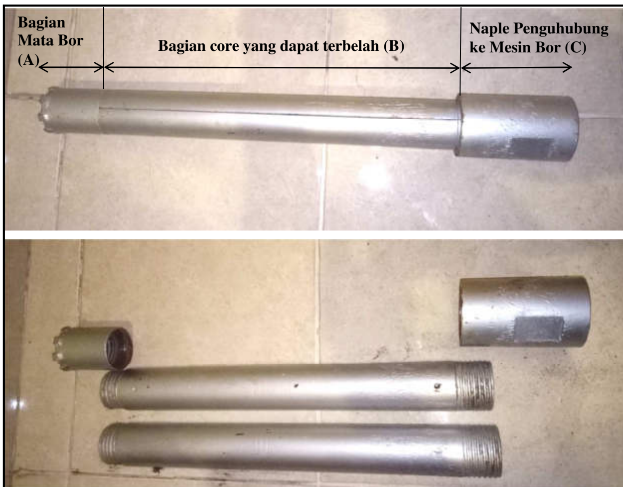
Gambar 3.3 Split Single core barrel / baru
